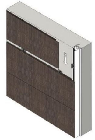
Installation of following panels Boiserie-H.
