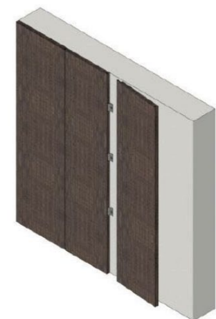
Installation of following panels Boiserie-V.
