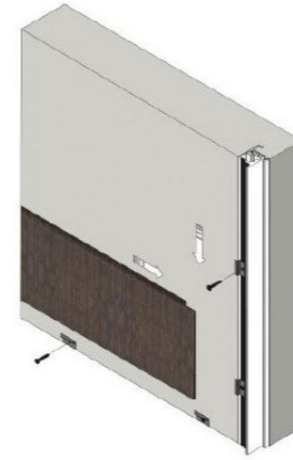
Installation of the starting panel Boiserie-H.
