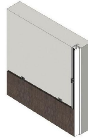
Anchor of the starting panel Boiserie-H.
