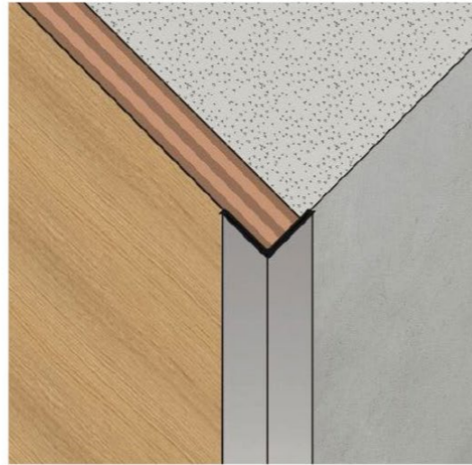
Matched or lacquered aluminum profile for closing.
