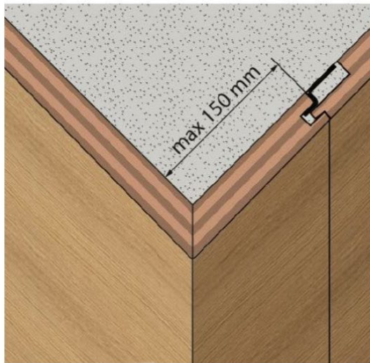
45° assembled panel with one side maximum dimension 150 mm.
