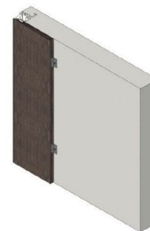
Anchor of the starting panel Boiserie-V.
