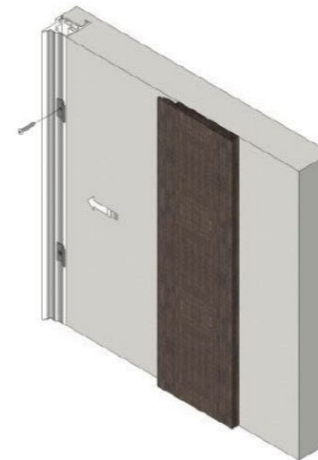
Installation of the starting panel Boiserie-V.
