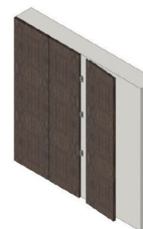
Installation of following panels Boiserie-V.
