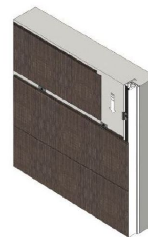
Installation of following panels Boiserie-H.
