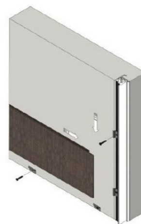
Installation of the starting panel Boiserie-H.
