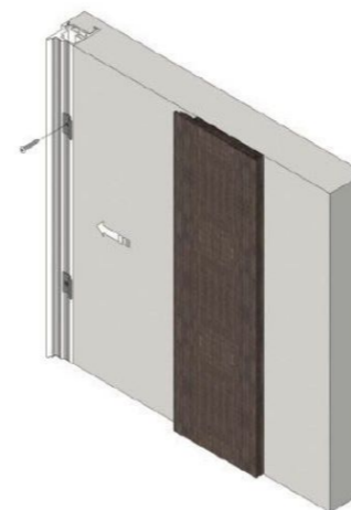
Installation of the starting panel Boiserie-V.
